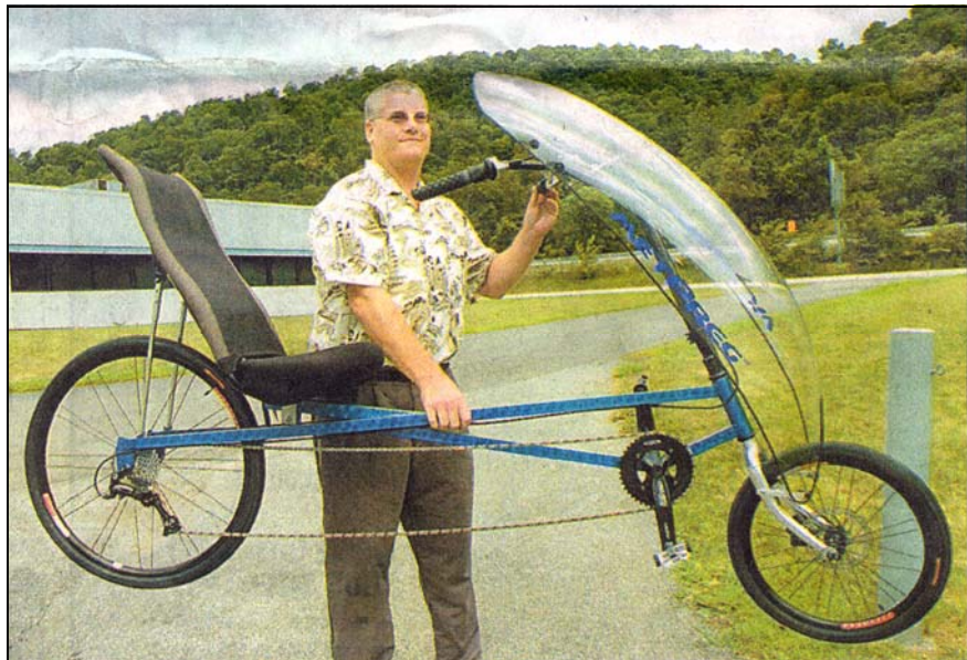
Gregg Wolfe, technical director for Touchstone, lifts the bicycle with a frame that weighs about 4 pounds, demonstrating that MetPreg can help make a variety of products light but strong.
