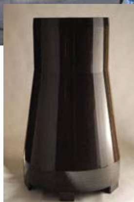
CFOAM composite tool for missile body application.
